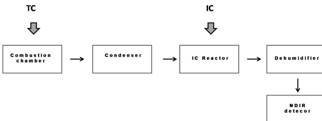
Fig. 5: Schematic figure of the TOC analysis.
