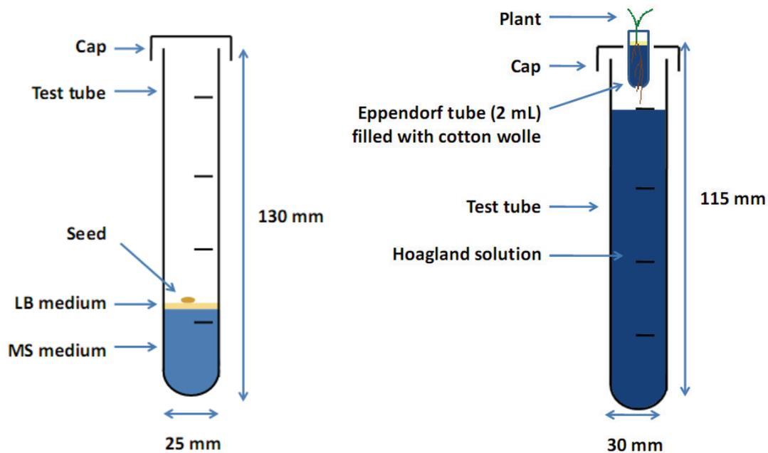
Fig. 6: Schematic figures of a growing tube (left) and the blue cap-system (right) for sterile plant cultivation.
